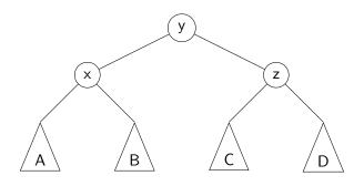
Notice that if heights of A, B, C, D differ by at most 1, then the tree is a proper AVL tree.
